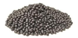
**XyloX™** is a revolutionary form of Thermoplastic Elastomer made entirely from 100% recycled tire reprocessed rubber crumb and recycled plastic pellets. The proprietary compounding process uses crumb rubber, post-consumer and post-industrial plastic pellets to create a molecular bond of the polymer chains. This is accomplished without the use of additional bonding agents providing a consistent and repeatable material.
